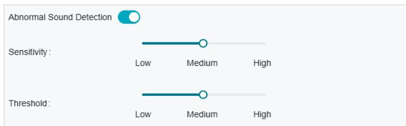
3. Adjust the value of sensitivity and alert threshold. The higher the sensitivity and the lower the threshold, the easier it gets to trigger linkage methods.
